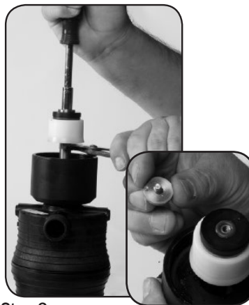
Step 2. Unscrew to unlock and remove #93 CAPSCREW.
