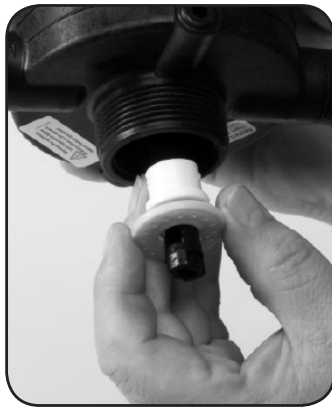
Step 7. Re-install #16 GASKET and #82 SEAL SPACER
