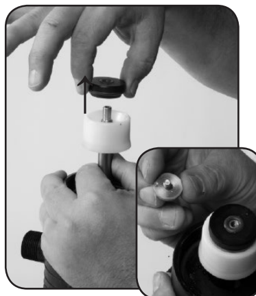
Step 8. Replace #73 DOSAGE PISTON GUIDE and #44 DOSAGE PISTON.
