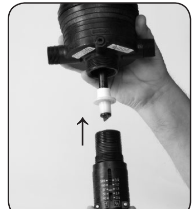
Step 9. Screw #7 OUTER CYLINDER onto body.
