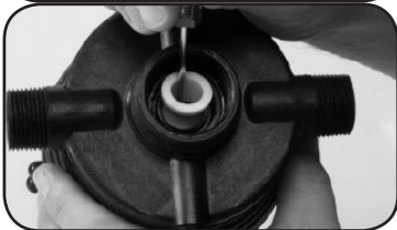
Step 4. Remove and clean #16 GASKET and # 82 SEAL SPACER.
