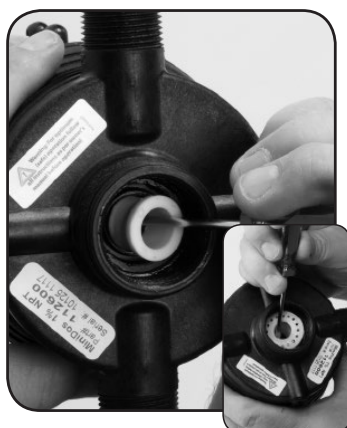
Step 7. Replace #82 SHAFT SEAL SPACER and #16 Gasket.
