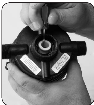
Step 4. Remove #82 SHAFT SEAL SPACER.
