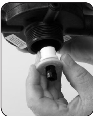
Step 7. Re-install #82 SEAL SPACER and #16 GASKET.
