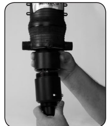
Step 9. Screw #61 OUTER CYLINDER onto body.
