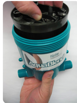
Step 6. Place new motor piston carefully into pump body and replace lid.
