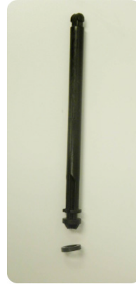
Step 3. Remove shaft with gasket and install new. If damage on sealing surface of shaft, replace shaft.
